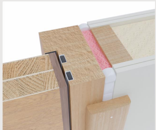
Image B – FD90 & FD120 foam with intumescent acrylic sealant cap of 10mm minimum.
